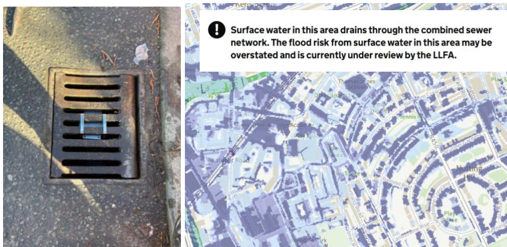
Gully sensor and revised surface water flood map with warning flag
