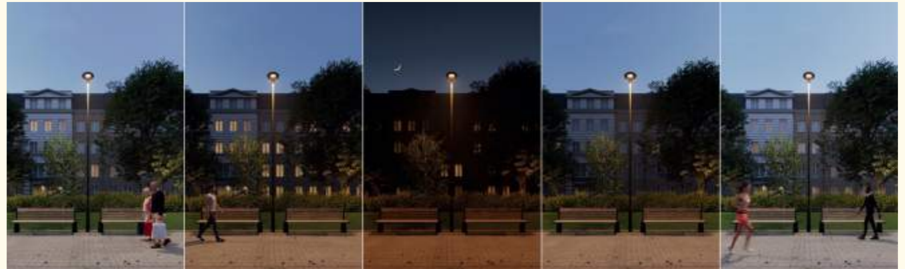
Early evening Pre-dawn Overnight Late evening Dawn 2,700K 2,500K 2,200K 2,500K 2,700K 100% Intensity 75% Intensity 75% Intensity 75% Intensity 100% Intensity
