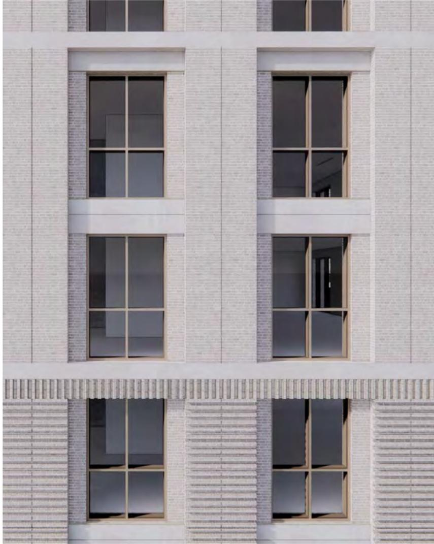
Fig 3.44: Example of vertical pier expression & facade layering
