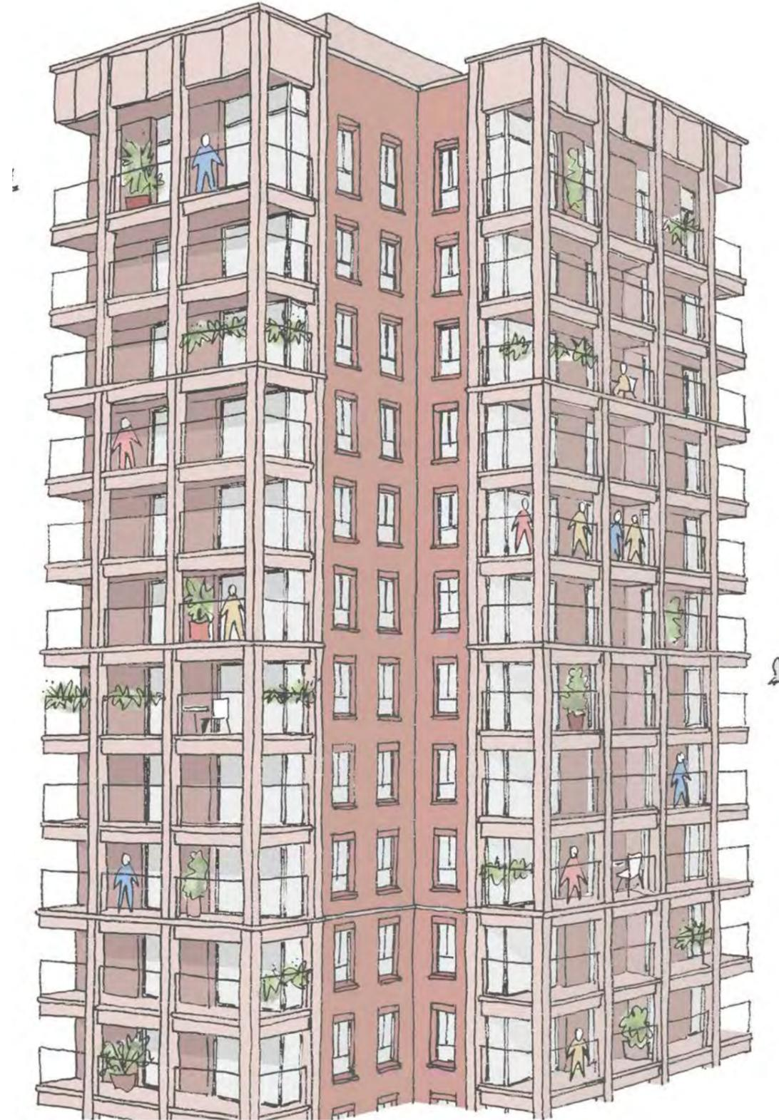
Fig 5.42: Plot 4.1 - Sketch of the towers ordered fenestration pattern and loggias
