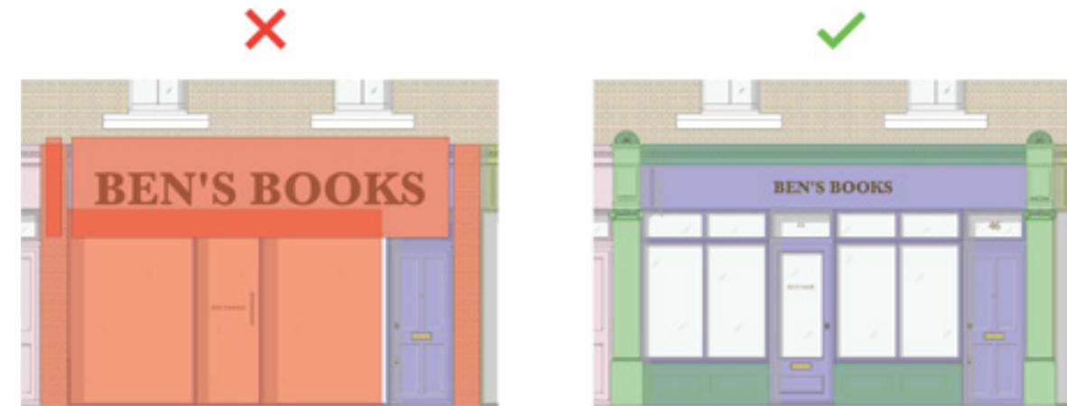
1.1 Retain and restore historic features
