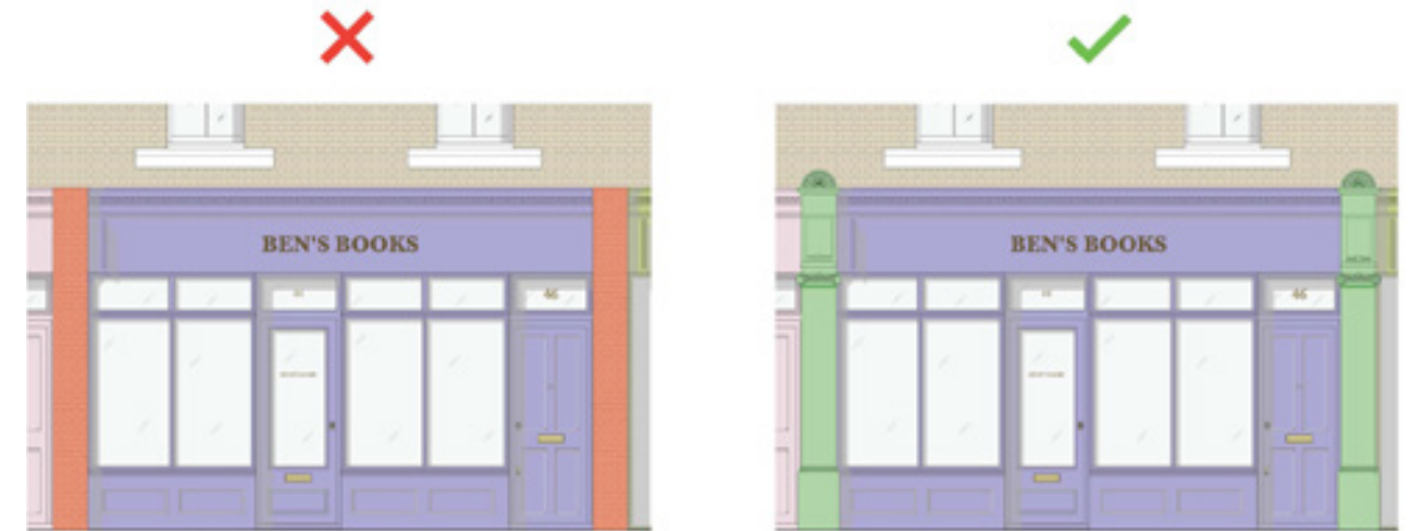
4.1 Restore pilasters and corbels
