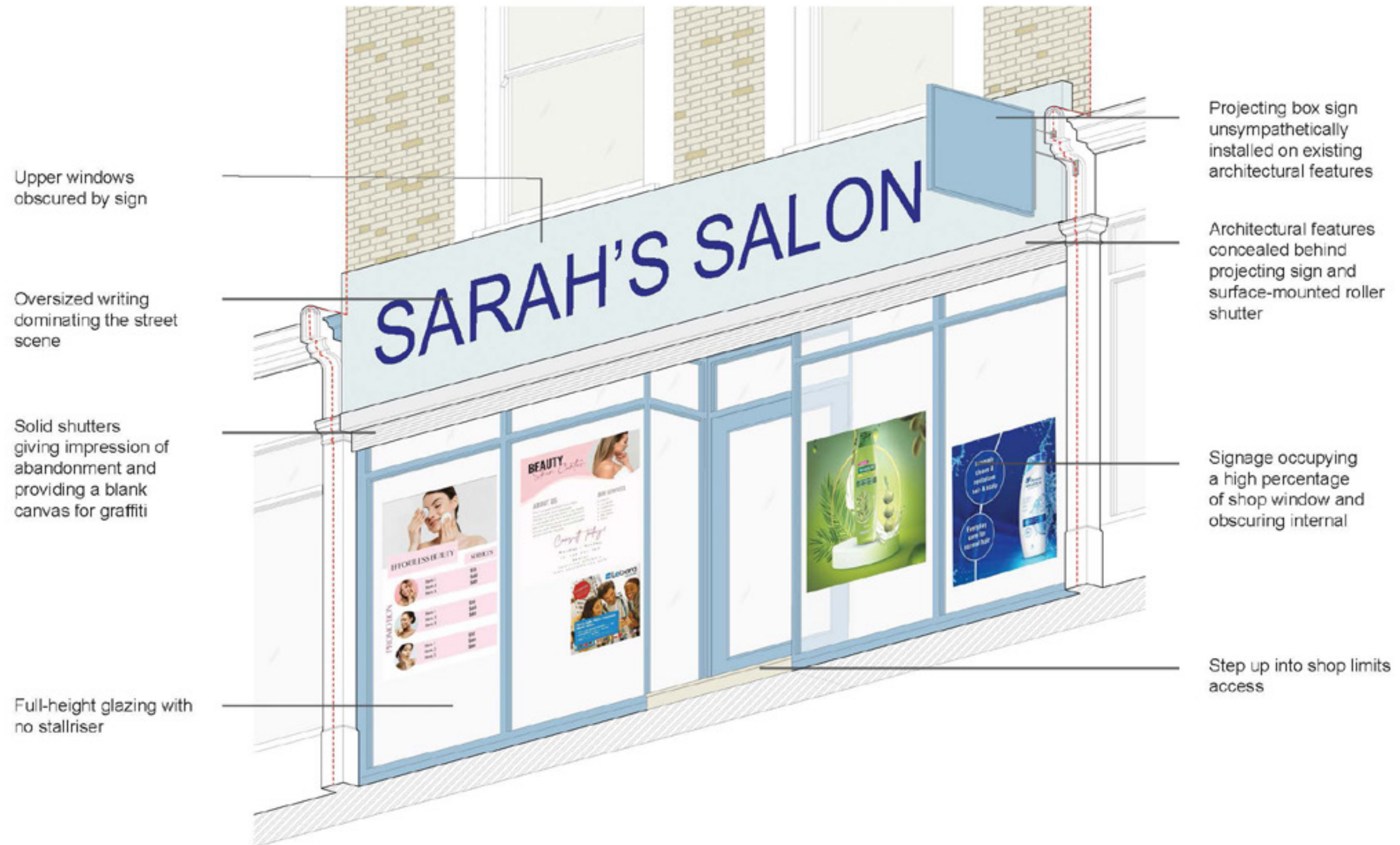
Negative example of a shopfront
