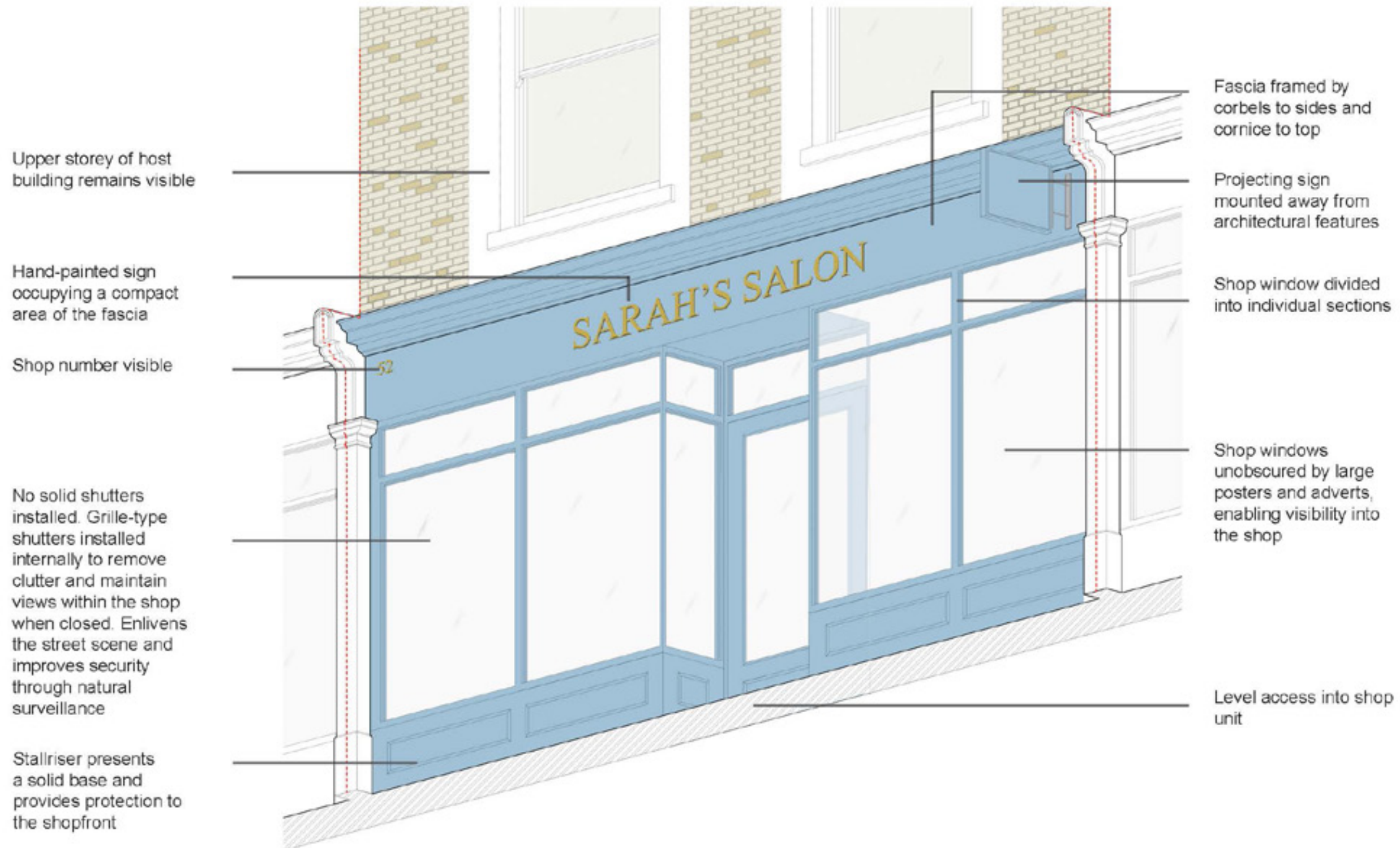
Positive example of a shopfront
