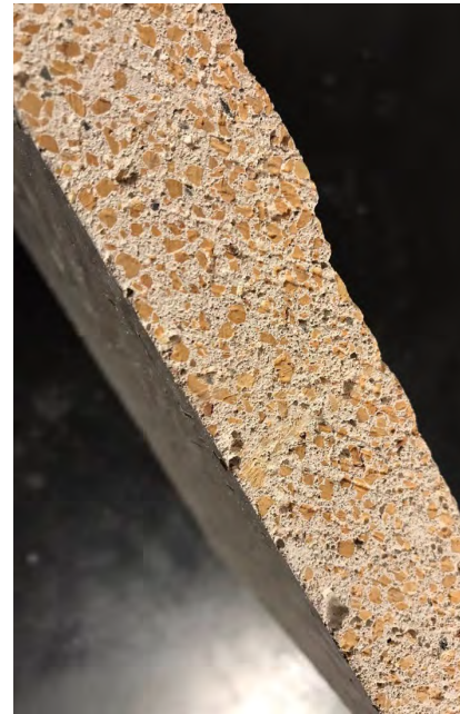
Cork granules visible in lime/cork plaster internal plaster insulation
