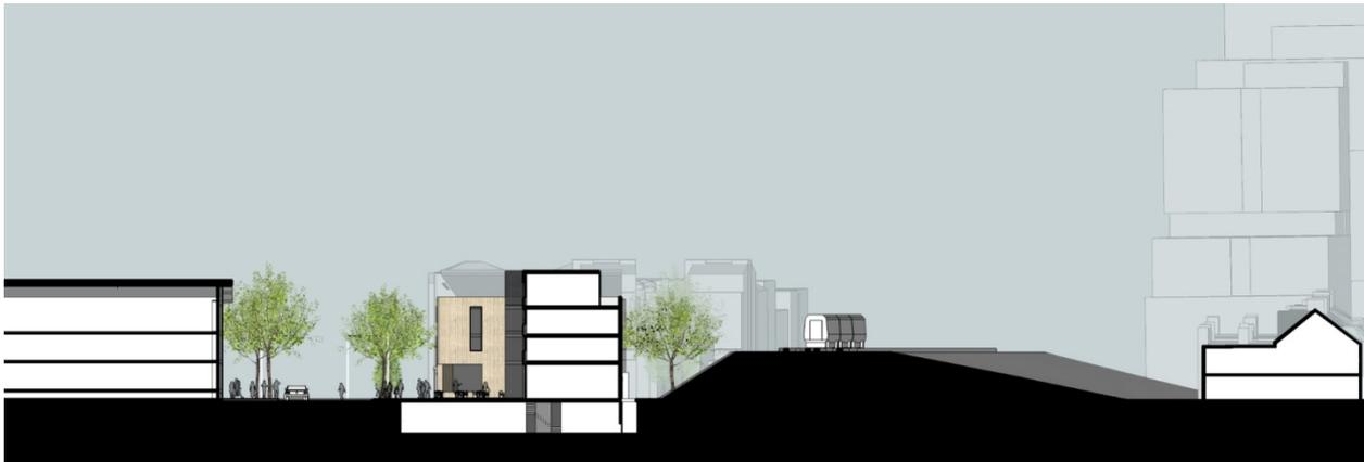
*Section through Latimer Road, railway line (Borough boundary) and Eynham Road showing height levels assuming redevelopment of Units 1-14 under StQW Draft Policies. Building shown on the eastern side of Latimer Road (to left of image) is the existing mixed use development at Nos 290-294.*
