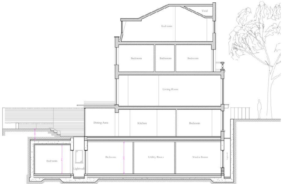
**Figure 3 Typical cross section of a basement extension**
