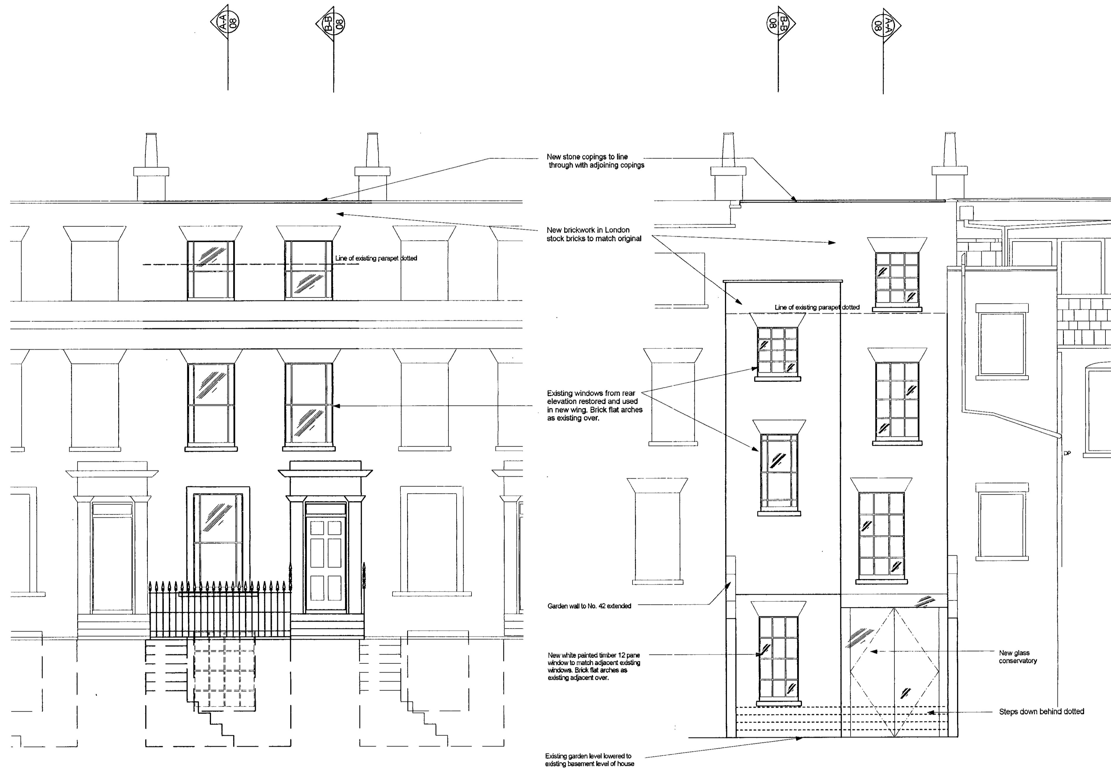
Front Elevation Restore all windows Clean down existing brickwork and repoint where necessary
