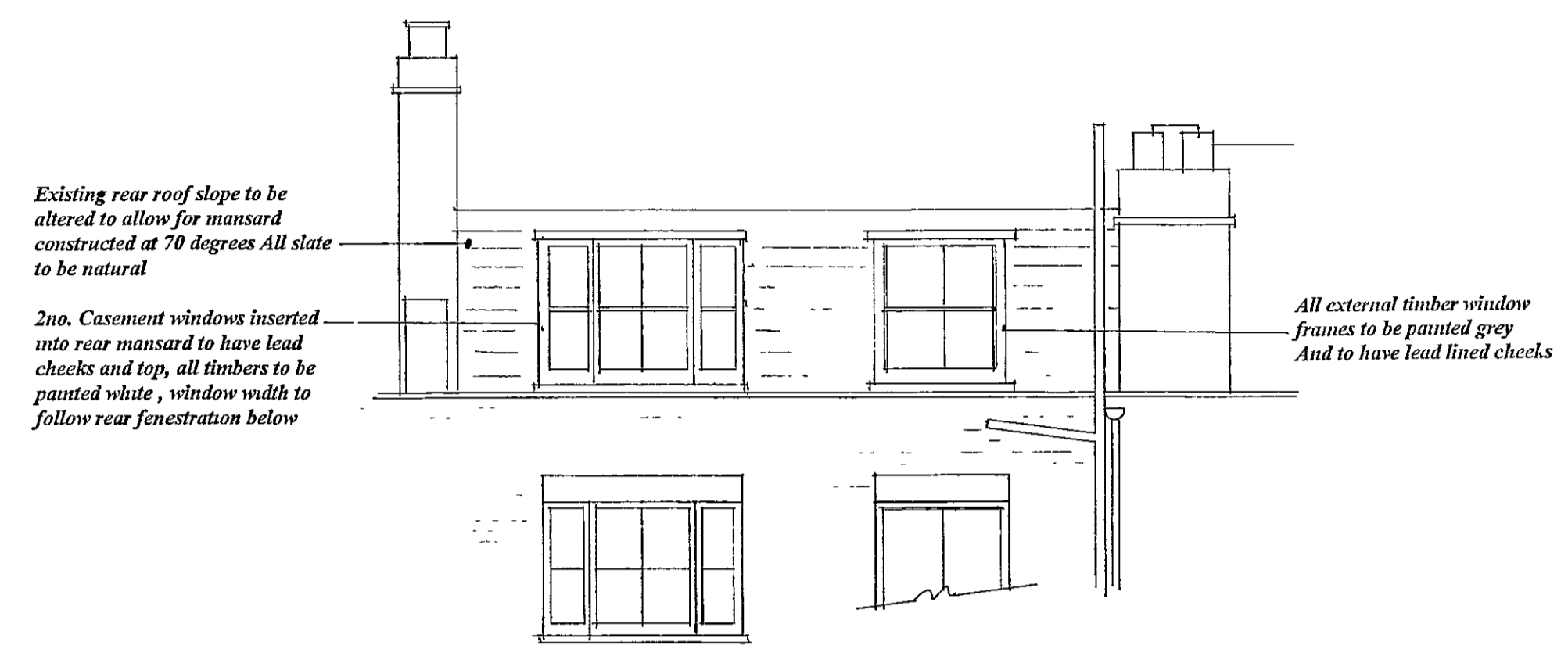
Proposed Rear Elevation at Roof Level
