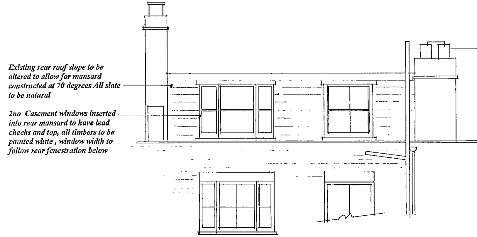
Proposed Rear Elevation at Roof Level
