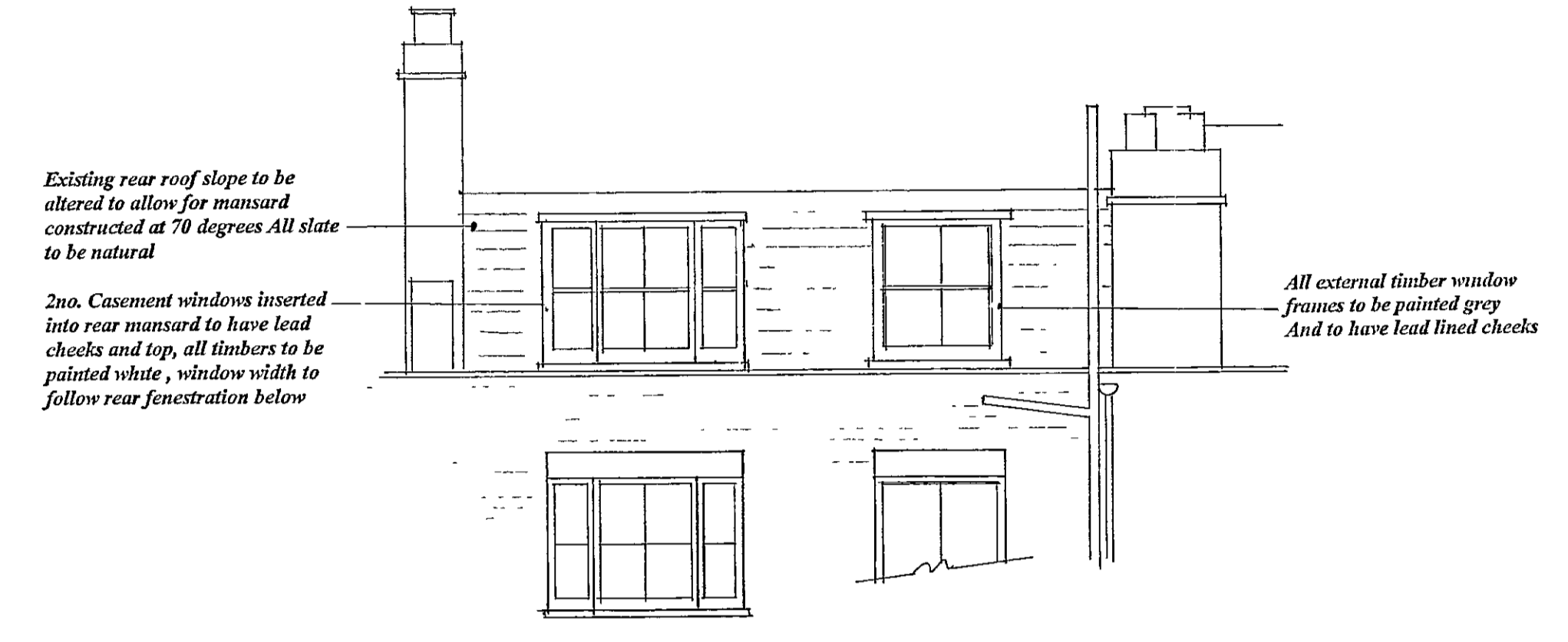
Proposed Rear Elevation at Roof Level
