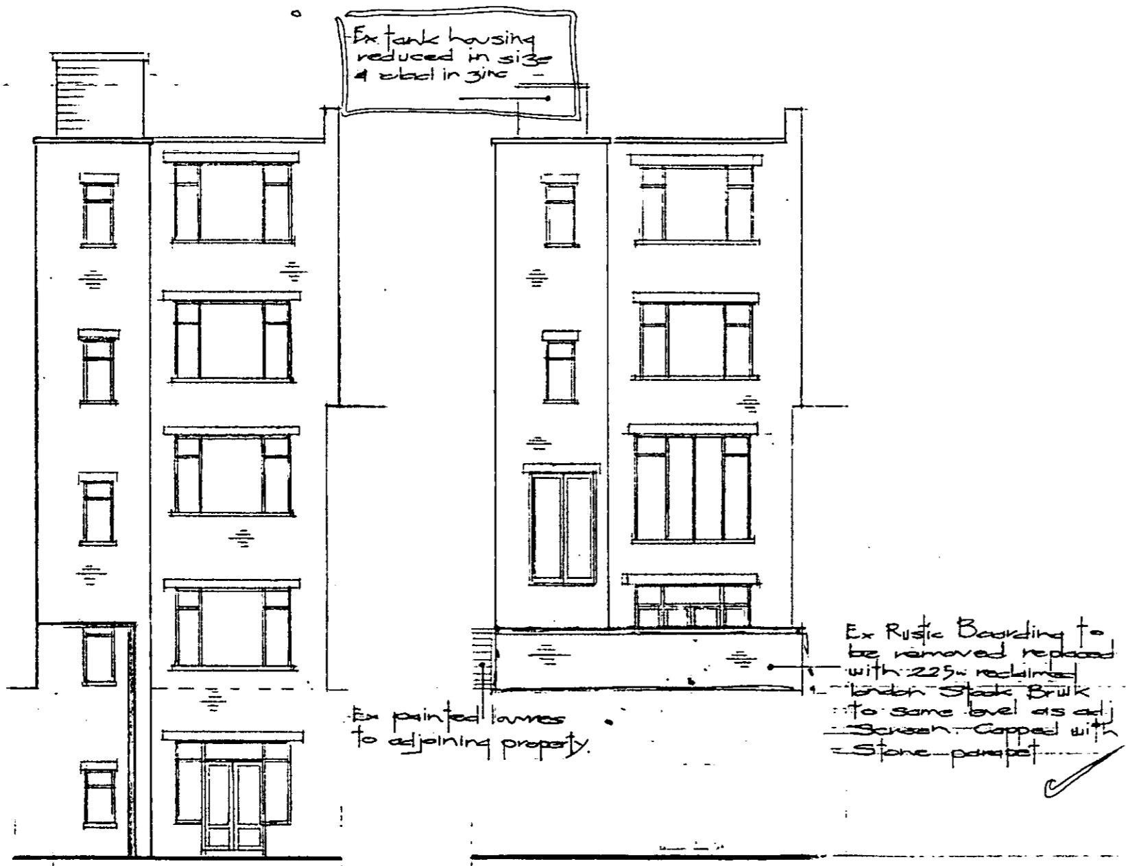
Rear Elevation Existing
