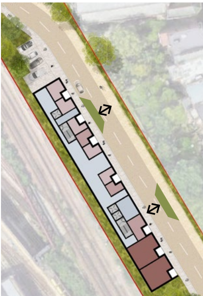
Design study illustrating the potential for a further reduced road width at select locations for traffic calming.
