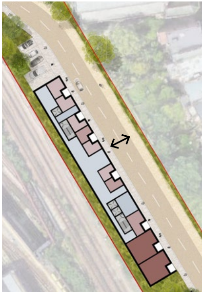
Design study illustrating a double lane road reduced to a 6.5m road width.
