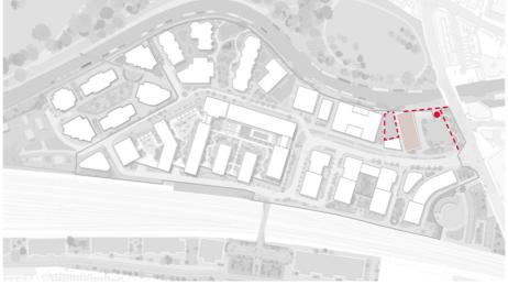
Fig 11.1: Plot 6 key constraints - Existing basin, water tower, gas line and level changes
