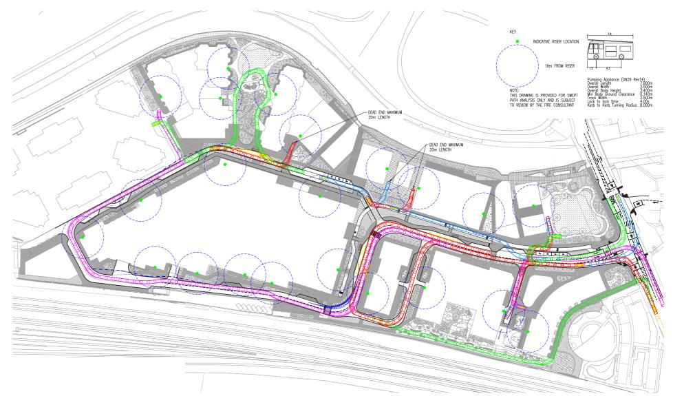
Fig 12.7: Diagram showing Fire Tender Tracking across the masterplan
