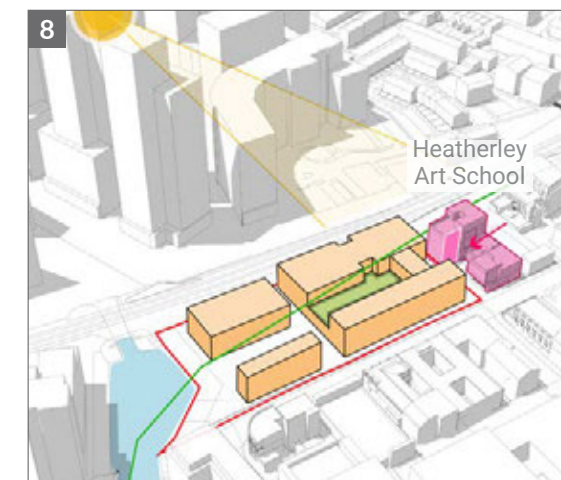
8 Considering pull back massing: Further adjustments to the massing are made to create more breathing space for the Heatherley Art School and to ensure they have sufficient daylight for their various classes
