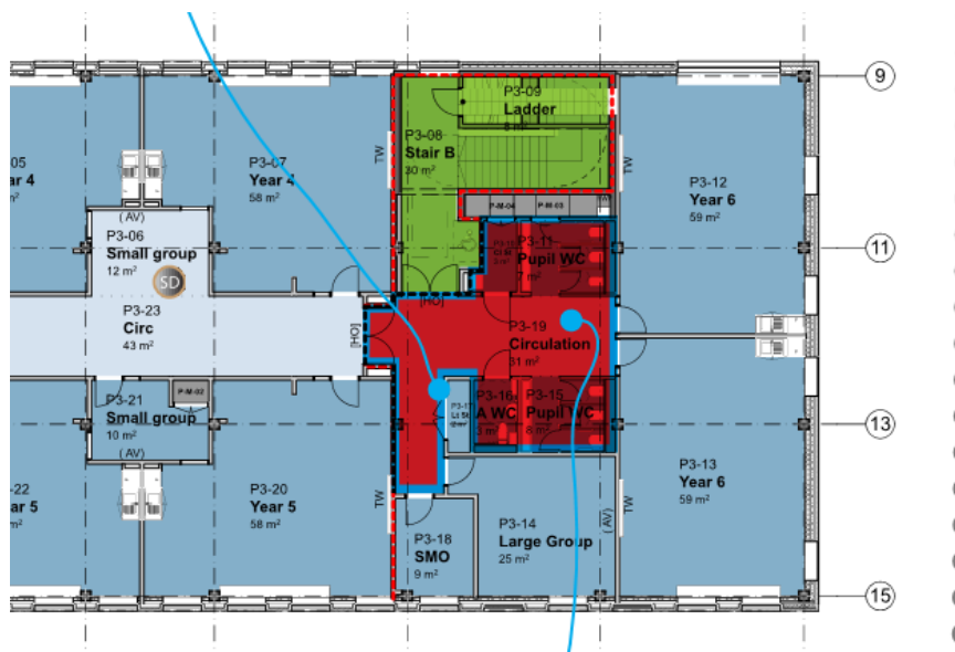
Figure 2. Dead-end corridor at Second Floor in the primary school which will be provided with a minimum of 30 min fire resistance to walls and FD20S fire doors.
