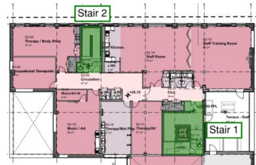
Figure 22. First Floor stair cores.
