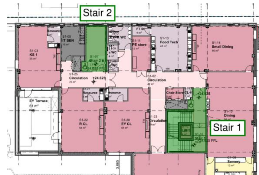
Figure 23. Ground Floor stair cores.
