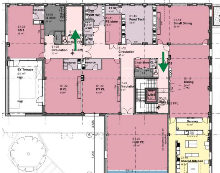
Figure 17. Storey exits at Ground Floor of SEN school.
