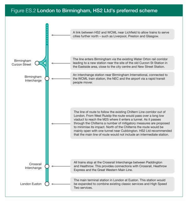
As described by HS2 Ltd, this route would run in tunnel from a rebuilt Euston Station, surfacing in West London to follow the route of the existing Chiltern Line, leaving London near Ruislip. The route would proceed largely in tunnel from the M25 as far as Amersham, and then continue to the west of Wendover and Aylesbury, partly in tunnel and partly following the existing A413 and Chiltern Line corridor.
