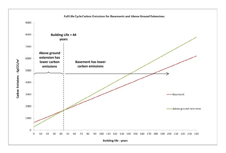
Further to this and as can be seen in the above graph it can be concluded that the subterranean and above ground extensions have the same total carbon emissions after **44 years**.
