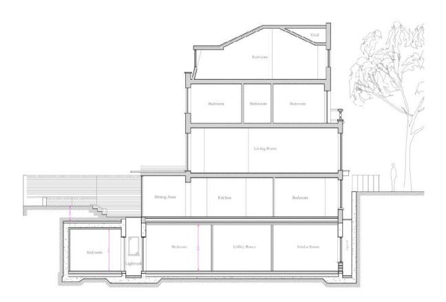
Figure 3 Typical cross section of a basement extension
