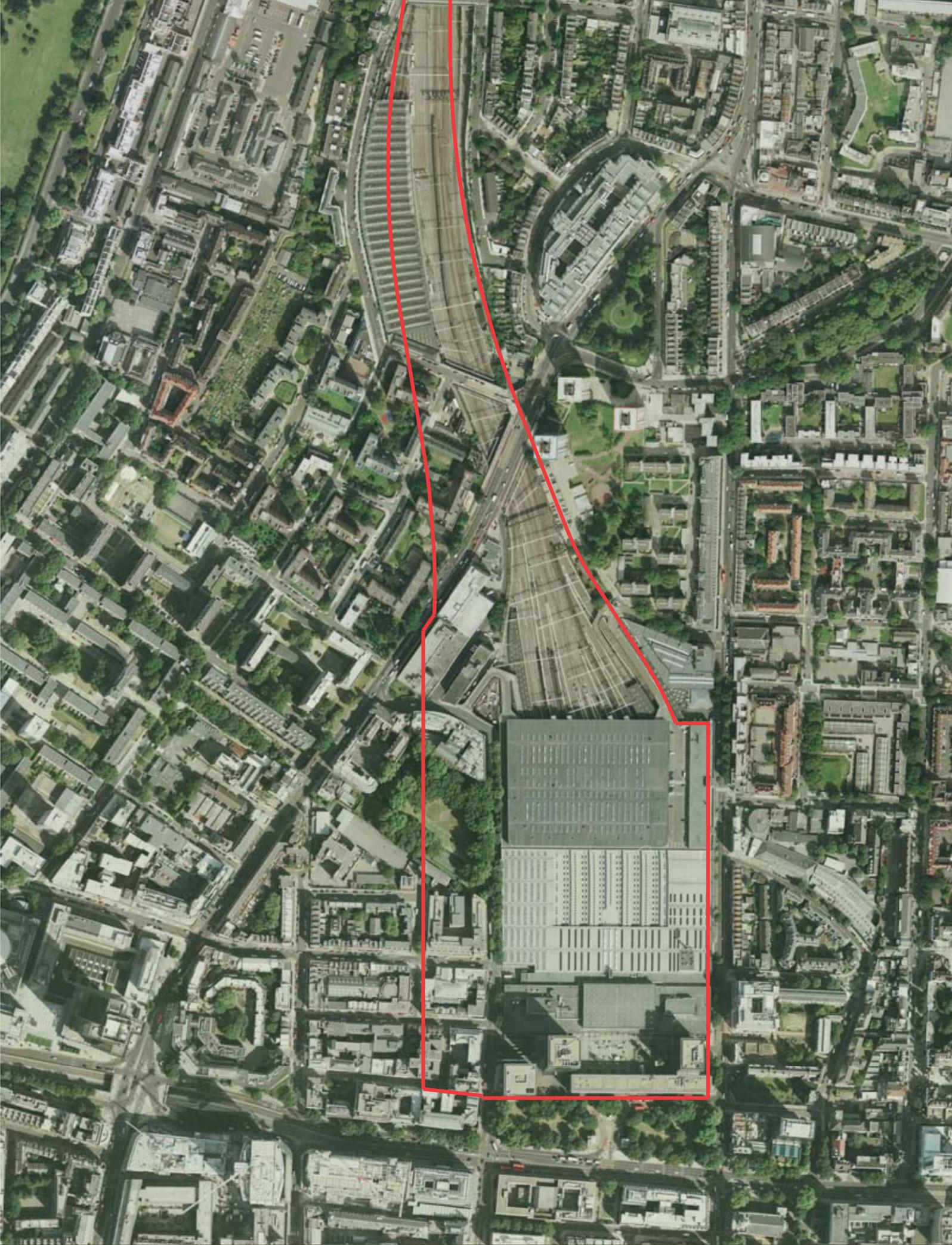
Proposed footprint of expanded Euston Station, to accommodate high speed and conventional trains
