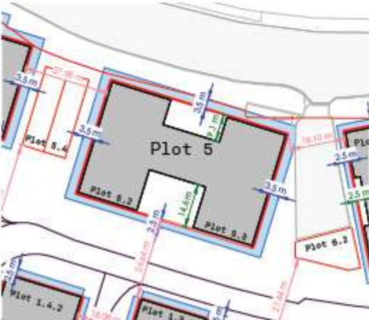
Fig 2.115: Plot 5 - Outline design parameters for plot 05 - showing a 3.5m zone for projecting balconies.
