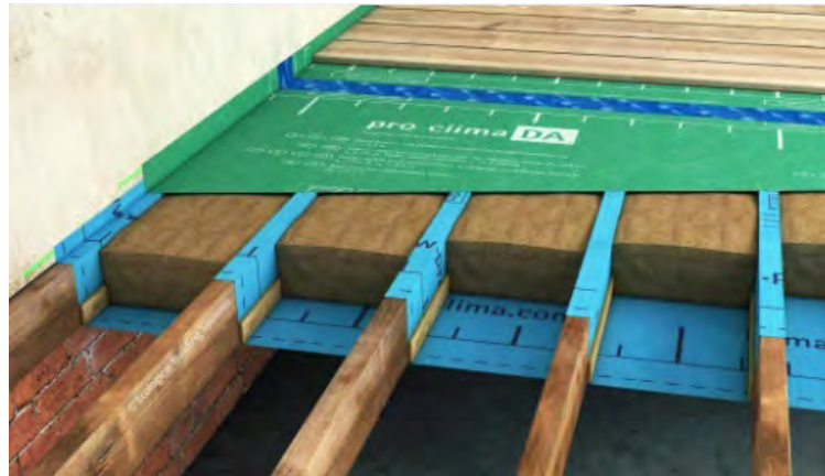
Insulated ventilated timber floor using hydroscopic insulation and breathable membrane – source: Ecological Solutions
