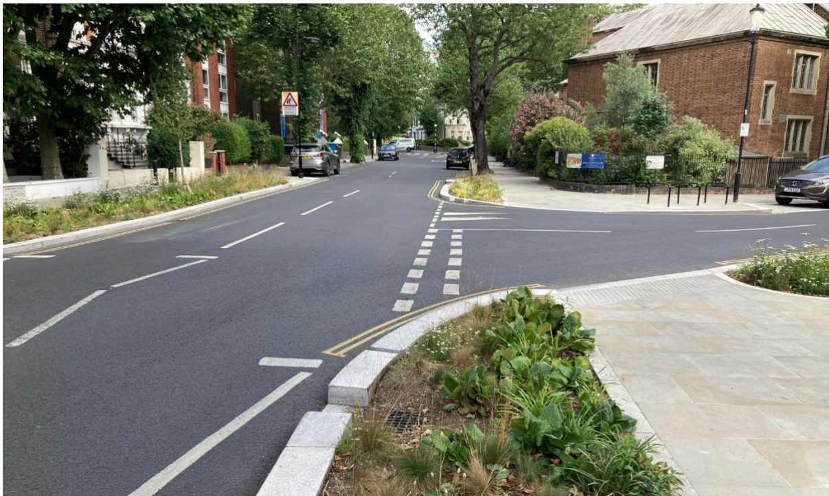
Rain gardens at the junction of St Helen's Gardens and St Quintin Avenue
