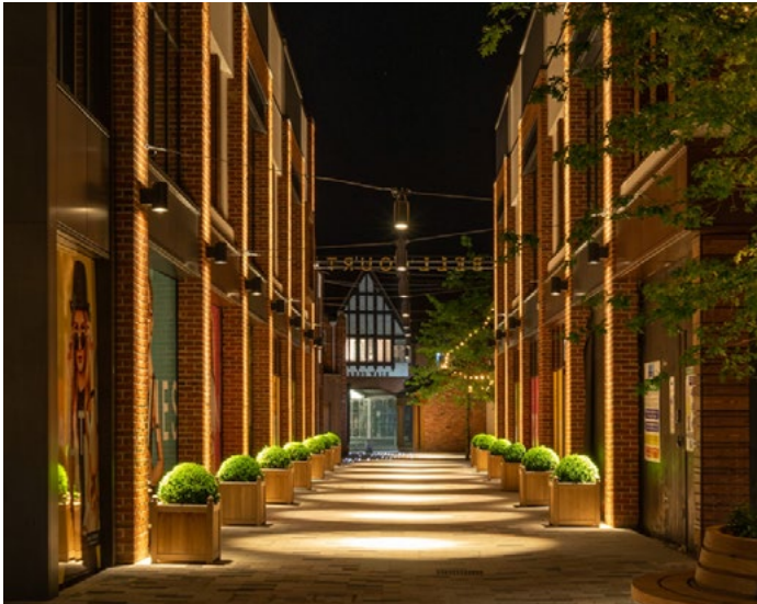
Catenary and building mounted light
