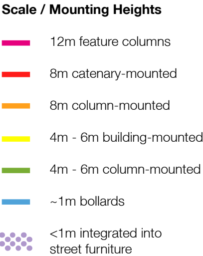
Mounting Height of luminaires application across Earls Court
